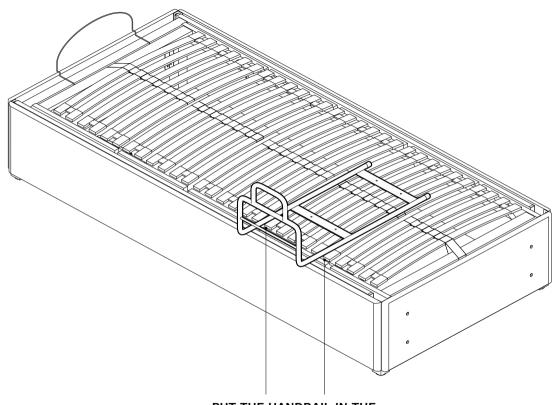
PUT THE HANDRAIL IN THE MIDDLE OF SLATS 5 AND 10
