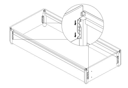
IF THE TONGUE OF ANY OF THE INTERLOCKING BRACKETS HAVE BECOME BENT, IT MAY BE NECESSARY TO USE A FLAT SCREWDRIVER TO LEVER IT OPEN TO ALLOW A GOOD FIT
