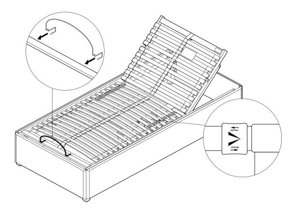
MORE FORCE IS EXCERTED IN THIS SECTION WHEN THE HEAD END IS RAISED. SLIDE THE TENSIONERS TO THE OUTSIDE TO MAKE THE SEATING SECTION FIRMER. THIS CAN BE SOFTENED IF REQUIRED BY SLIDING THE TENSIONERS TOWARDS THE MIDDLE
