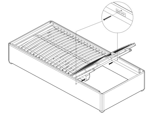
SECURE THE MECHANISM TO THE BASE USING THE 2 X 40MM SCREWS SUPPLIED. IF THERE ARE NO LABELS OR PRE-DRILLED HOLES FOR THESE SCREWS, SIMPLY SCREW THROUGH THE PLYWOOD INTO THE BASE APROXIMATELY WHERE SHOWN IN THE DIAGRAM
