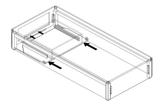
ENSURE THE BASE PANEL SITS ABOVE THE FOOT END SUPORT BATTEN AND HARD UP AGAINST THE FOOT END PANEL.IF THERE IS A GAP ON EITHER SIDE, CHECK THE BASE CORNERS ARE SQUARE (SEE PAGE 12)
