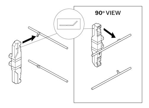
ALIGN THE MOTOR WITH THE HOOKS OF THE DRIVE BAR ENSURING THE HEAD END OF THE MOTOR MATCHES THE HEAD END BAR OF THE MECHANISM
